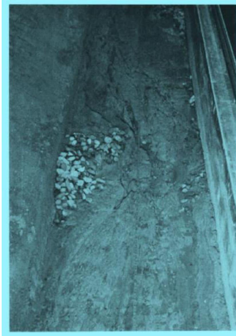
Figure 12. Channel three, localization of scour with respect to bend constriction.
