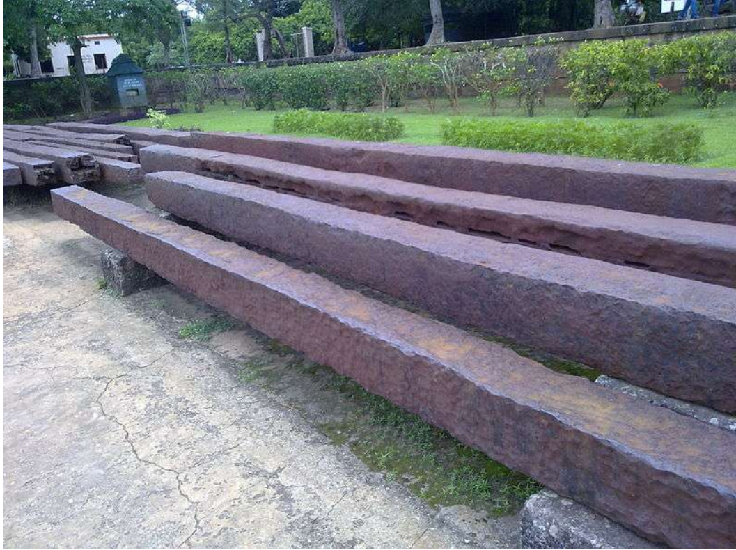
Another surviving example of ancient iron metallurgy is the Iron Beam at the Konark Temple premises.
