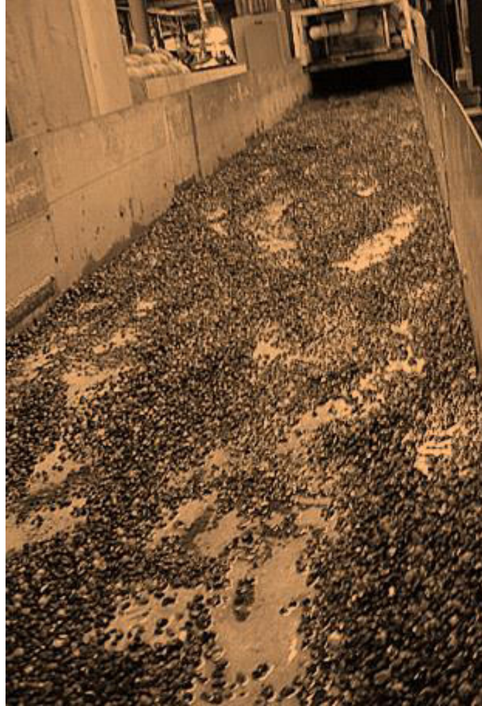
Figure 6. An example of gravel patches placed before commencing runs simulating an initial state with sediment from landslides. This configuration was used for all runs with slopes less than 0.015, except series 2-Ax and 2-Dx-a to e, which began from a bare bed. For all runs with slopes greater than or equal to 0.015, the runs were commenced with a complete alluvial cover with uniform thickness ranging from 1 to 6 cm. For Run 2-Bx, the run began from a bare bed.
