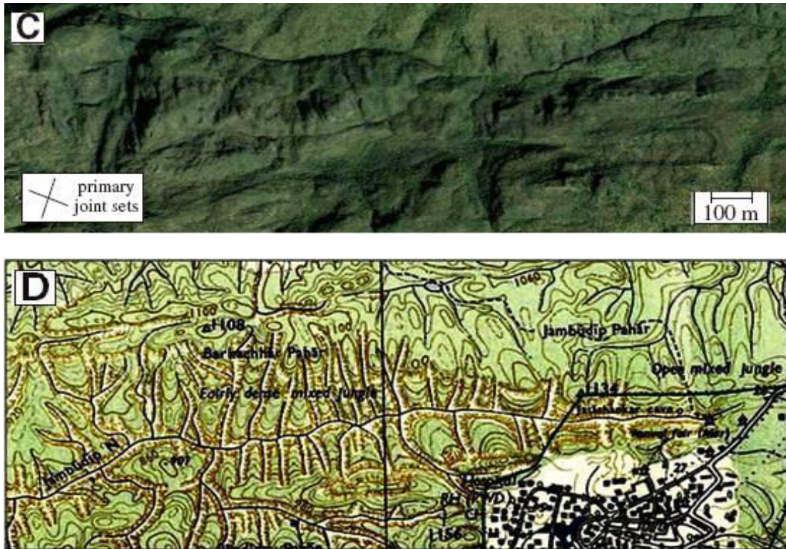
Figure: 8. Aerial photographs illustrating, examples of the correlation between joint and orientations locally. In each image, primary joints sets were identified by measuring the orientations of bedrock fractures visible in the photographs. This approach assumes that weathering and slope failure take place preferentially along joint sets, a hypothesis that is strongly supported by field observations. River lines highlight the locations where the local channel orientation closely aligns with one of the two primary joint sets. (A, B) The orientation of the primary joint sets is within 15^\circ of the regionally averaged joint orientations, which, in turn, closely match with the extension-parallel and extension-perpendicular directions. (C) The primary joint sets are displaced \sim 45^\circ counterclockwise from the regionally averaged orientations. (D) Part of toposheet 55J/7 depicting the Jambudip River and steep slope structure.
