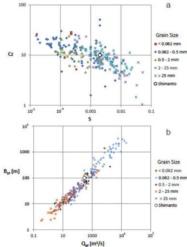
Figure 8. (a) Chezy resistance coefficient  $Cz$  plotted against bed slope  $S$  for alluvial rivers. Also included are estimated values for the Wainganga River, India. (b) Bankfull width  $B_{bf}$  versus bankfull discharge  $Q_{bf}$  for alluvial rivers. Also included are estimates for bank-to-bank width and characteristic flood discharge in the Wainganga River, India. The ranges for characteristic bed material size of the alluvial rivers are denoted in the legends.
