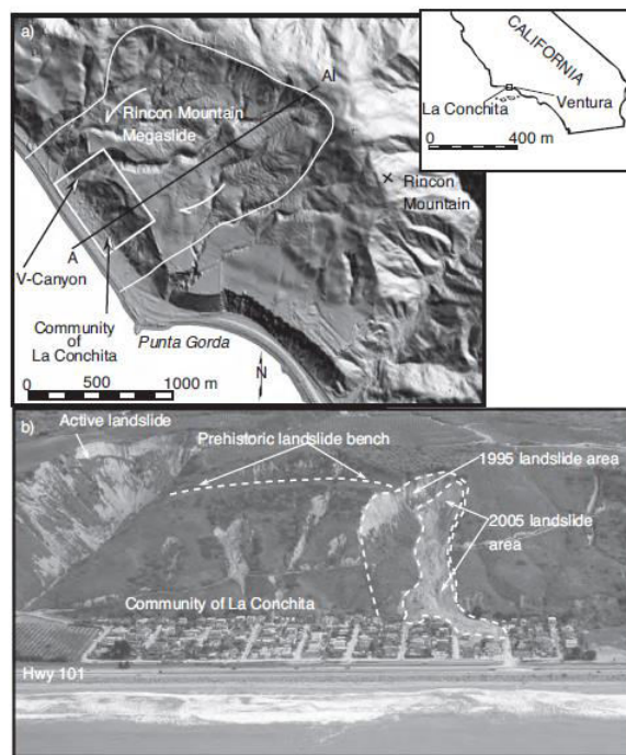
Figure .4 Interpretation of LiDAR/aerial imagery to recognize multiple ages of landslides above La Conchita, California, including a prehistoric landslide that lay unrecognized during the development of the community of La Conchita (from Gurrola et al., 2010)
