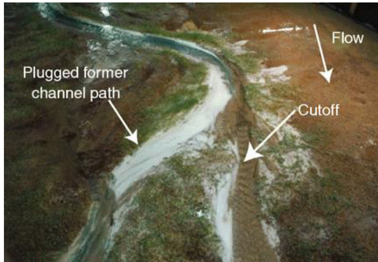
Figure 5. Photograph of cutoff channel and fine sediment filling the first channel. Sediment colours are the one as Fig. 3. Fines comprised the downstream end of the bar seen in the photograph. This was the final cutoff of the experiments and was caused by headward erosion rather than bar migration into a chute.
