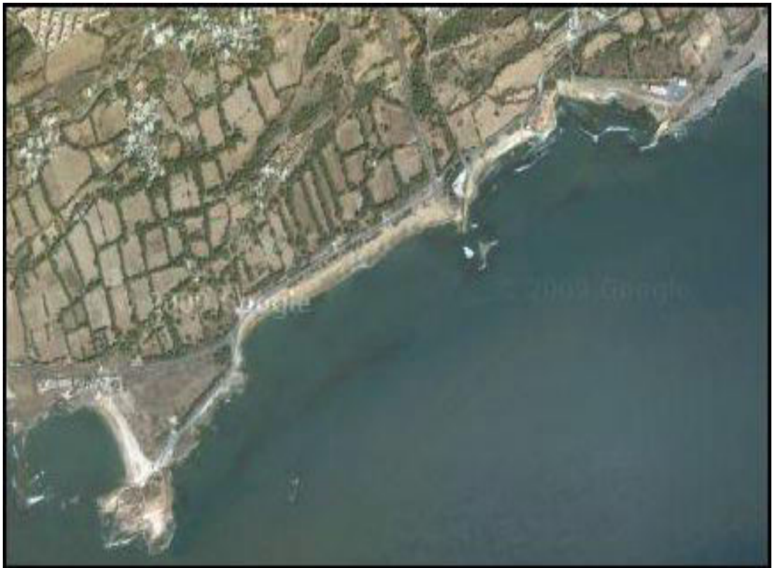
Figure: 20 The beach must be free to align itself parallel to the direction from which the refracted waves reach the foreshore. (Google earth Photography)
