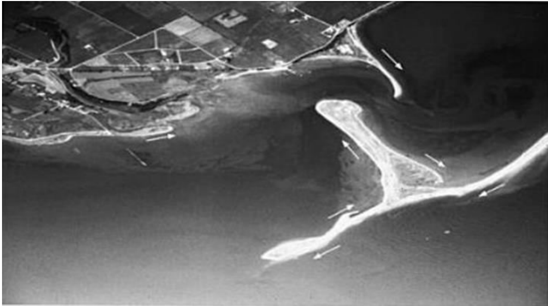
Figure:14 Diu Spit in the Arabian sea, with arrows indicating the directions of Long shore drifting, determined by local exposure to wind-generated waves. (Google earth Photography)
