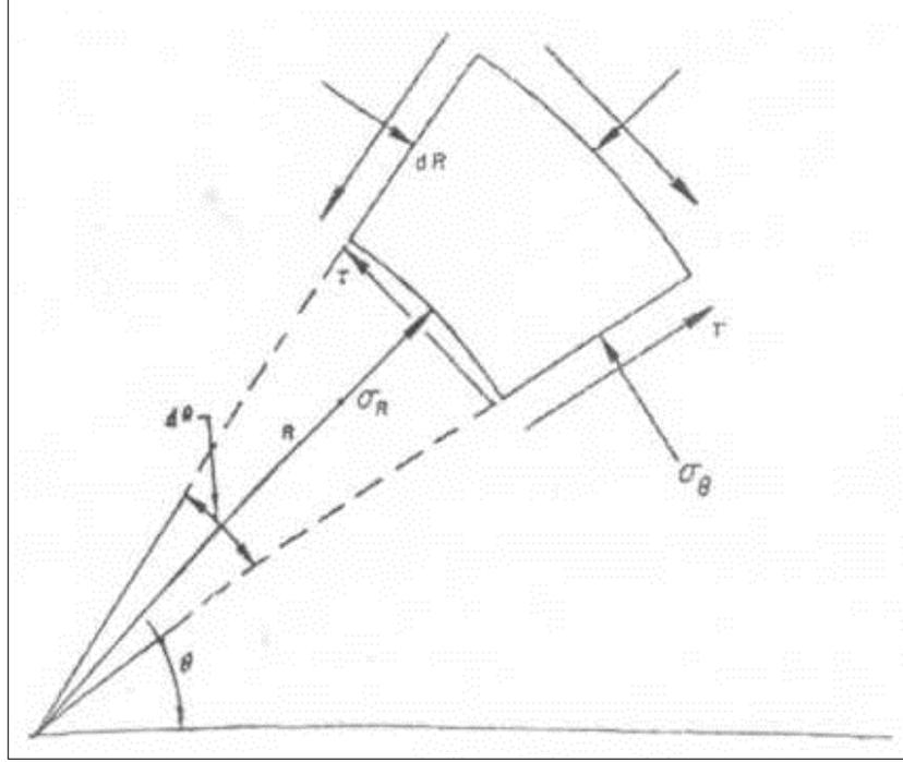
Figure. 3 – Stresses acting on a small element of Volume.
