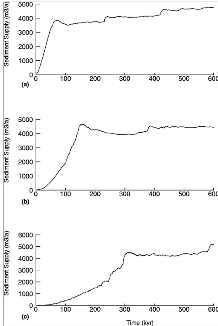
Figure 7. Sediment supply versus time for catchment X indicated in the model shown in Figure 2 in model runs with a range of values of the critical threshold (a) 2.5, (b) 5.0, and (c) 10.0  $m^{0.8}$ .
