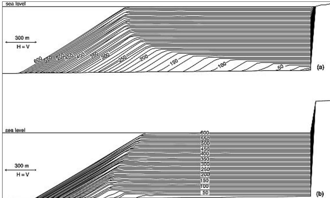
Figure 8. (a) Internal stratigraphy of fan deltas shown in a representative dip-oriented section through the delta fed by catchment Y. (b) Comparative internal stratigraphy of a delta developed under conditions of constant sediment supply. In both cases the stratigraphy is recorded/displayed at intervals of 12.5 kyr and highlighted every 50 kyr. No vertical exaggeration.
