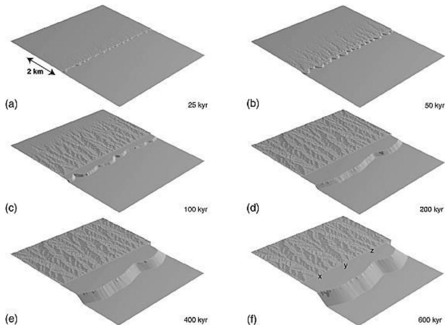
Figure 2. Progressive development of a model with repeated earthquake events producing 0.5 m of uplift and 1.0 m of subsidence every 1000 years over a total run time of 600,000 years. The value of the critical threshold for erosion used is  $5.0\text{ m}^{0.8}$ . All other model parameters as in Figure 1. No vertical exaggeration.
