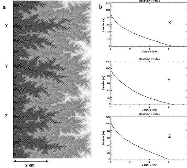
Figure 3. (a) Map view of footwall drainage basins at end of model run shown in Figure 2f. (b) Representative stream profiles for three catchments (labeled X, Y, and Z) developed on the landscape.
