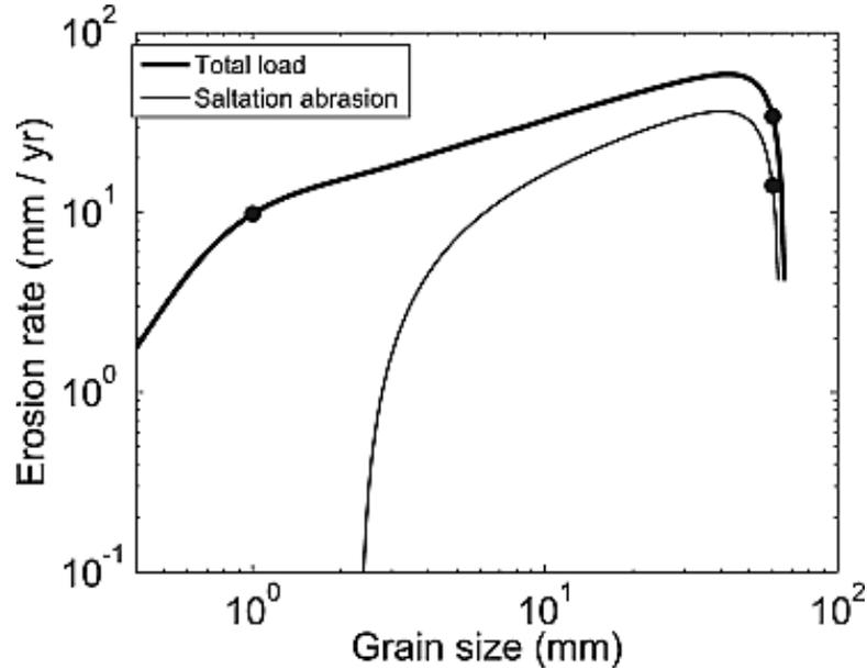
Figure 7. Log-log plot of erosion rate versus grain size for a constant flow depth ( $H = 0.95$  m), channel slope ( $S = 0.0053$ ), and sediment supply ( $8.9 \times 10^{-4}$  m<sup>2</sup>/s). The black circles are the conditions for the representative field case of the Nibra River (Table 1).
