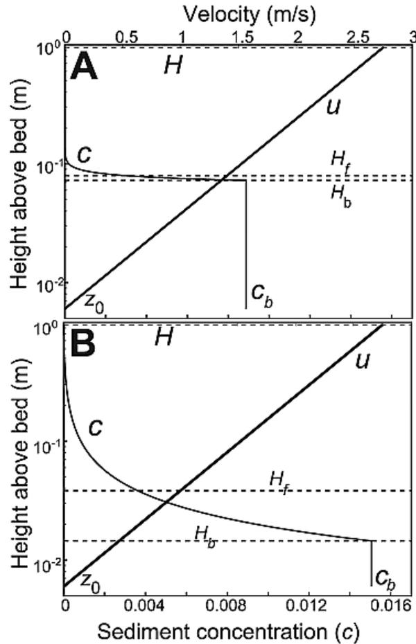
Figure 1. Schematic showing vertical profiles of sediment concentration  $c$  (equation (26)) and velocity  $u$  (equation (21)) for the conditions of the Nibra River (Table 1) and for (a) 60-mm gravel and (b) 1-mm sand. Also shown are the calculated heights of the bed load layer  $H_b$  (equation (25)), weighted average particle fall heights  $H_f$  (equation (32)), flow depth  $H$  (Table 1), and the near-bed sediment concentration  $c_b$  (equation (18)).
