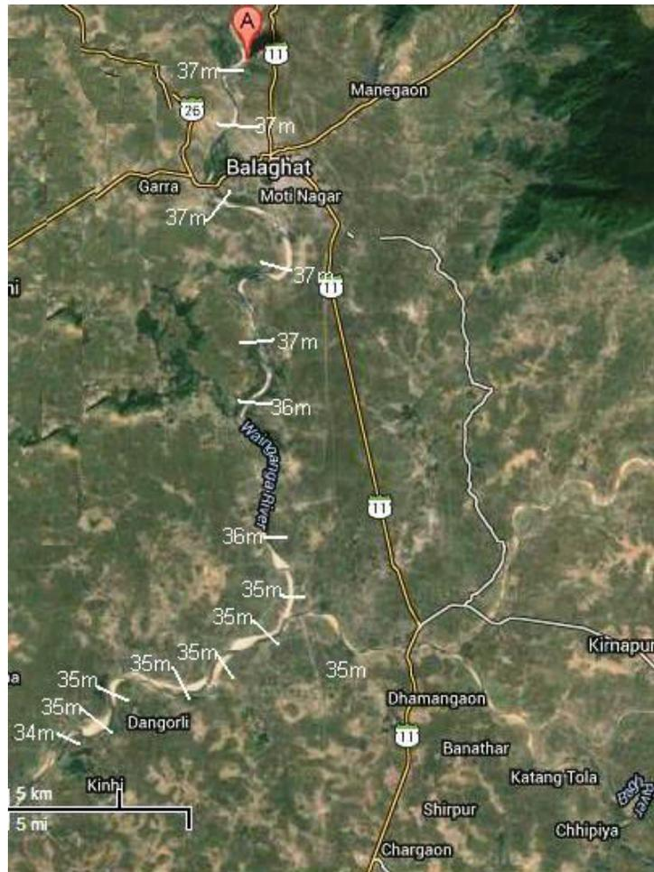
**Figure 5. Planform configuration of the investigated Wainganga river reach, including the confluences with the Bagh and Bawanthadi streams. The image has been downloaded from Google maps. The sections drawn in the figure are those recently surveyed by Dr N. L. Dongre (2014). The flow is from north to south.**
