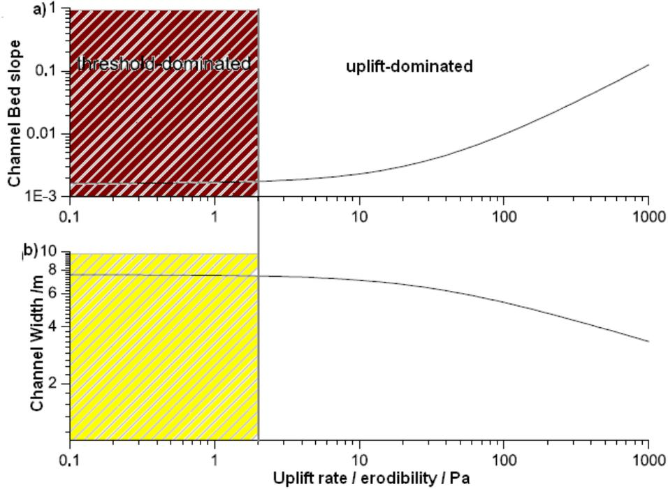
Figure 7. Functional form of (a) slope and (b) width response on tectonic uplift as predicted by equations (10) and (11) for a discharge  $Q = 50 \text{ m}^3/\text{s}$ . In the threshold-dominated domain both width and slope are approximately independent of uplift rate. Gray shading shows the approximate extent of the threshold-dominated region, and the gray line at  $U = 0.1 \text{ mm/a}$  shows the approximate boundary between threshold- and uplift-dominated domains.
