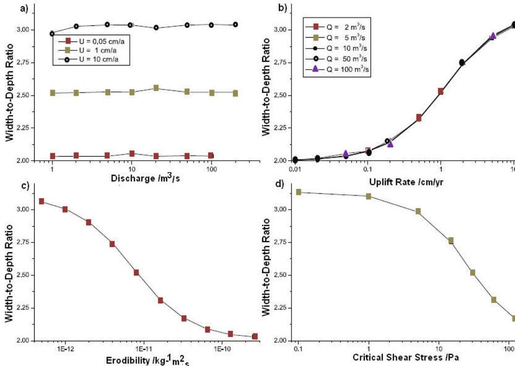
Figure 8. Width-to-depth ratio as a function of (a) discharge, (b) uplift rate, (c) erodibility, and (d) critical shear stress. The simulations for Figures 8c and 8d were done at  $Q = 50$   $m^3/s$  and  $U = 0.1$   $mm/a$ .
