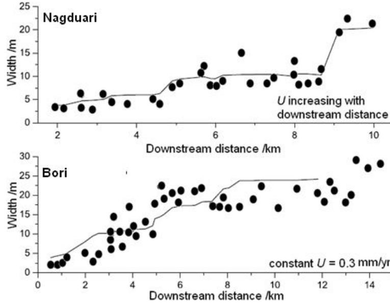
**Figure 3.** Channel width for the Bori of central Pachmarhis and the Dudhi Rivers, of Patakot. These two channels crossing active faults in the Pachmaris (data digitized ). While for the Bori, the uplift rate is constant in the direction normal to the fault (uniform block uplift), for the Dudhi it increases in the downstream direction. The solid line gives the expected channel width if it scales with the square root of drainage area (see equation (8)).
