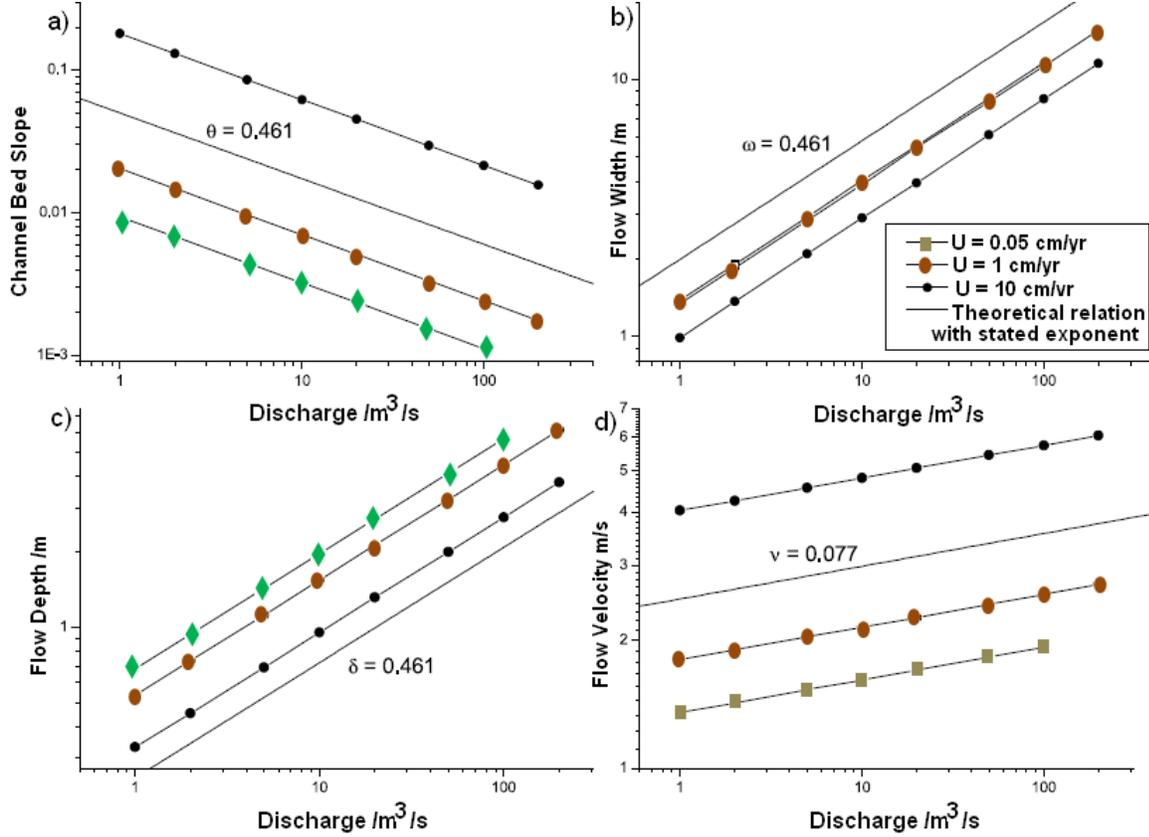
**Figure 5.** Steady state geometry parameters (a) slope, (b) width, (c) depth, and (d) velocity as functions of discharge for channels at various uplift rates. The power law exponents obtained from fits to the data are given on the plots for comparison (see equations (7)—(10), (17), and (18)).
