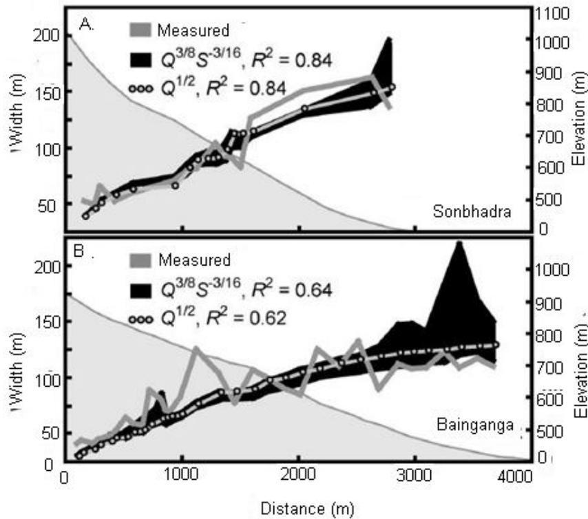
**Figure 3. Profiles on long River and comparisons of channel width. Channel width derived from a  $Q^{1/2}$  relationship, and channel width derived from equation 5 for Sonbhadra (A) and Bainganga (B). Uncertainties due to errors in width measurement and digital elevation model-derived river slopes are represented by line thickness.**
