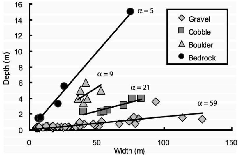
**Figure 3. Plot of  $\alpha$  for different dominant channel substrates. Gravel data are from Denwa River of Satpura, and largest bedrock width data point is from Sonbhadra River of Pachmarhis. Other data are from field surveys in the Pachmarhis region. While gathered from various locations, all bedrock data are from channels incised in high-grade Deccan Trap rocks.**
